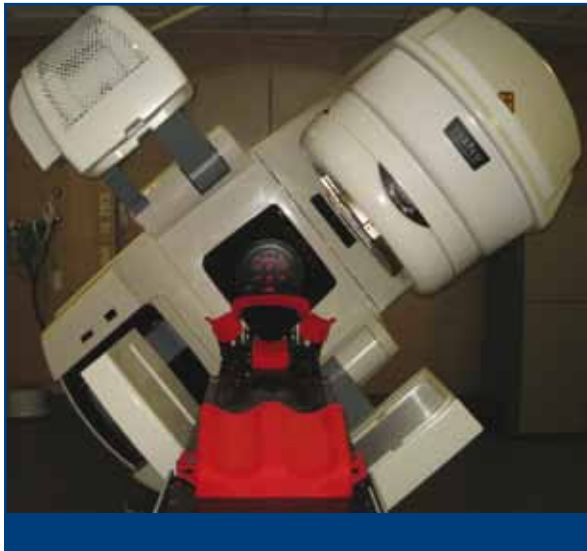
Figure 5. On-board imager (OBI, Varian®). X-ray tube and kV-flat panel imager mounted on the gantry of the linear accelerator, orthogonal to the MV source.
